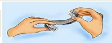
6 Similarly insert other rings and ensure that the joints are at 90°. N.B: rings must be fitted individually and not as a set
