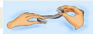
6 Similarly insert other rings and ensure that the joints are at 90°. N.B: rings must be fitted individually and not as a set
